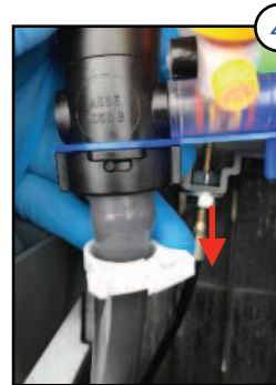
Declipser la bague grise
